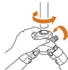
4. Insert the center column from the lower side of the main body and tighten the locking collar and the center base column base stopper.
